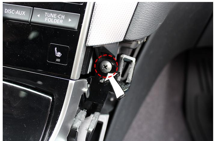
Unfasten **two (2)** Philips screws **one (1)** on each side beside heated switch.
