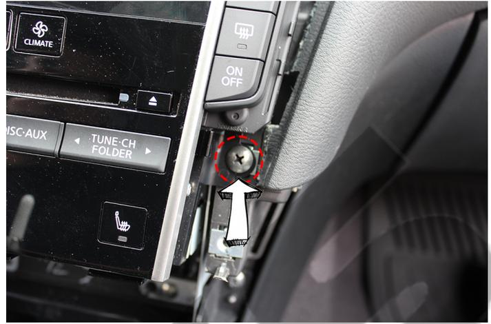
Unfasten **two (2)** Philips screws, **one (1)** on each side of the radio below the side buttons.
