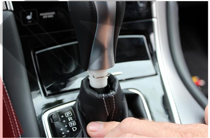
Pull down shifter boot to expose shifter pin.
