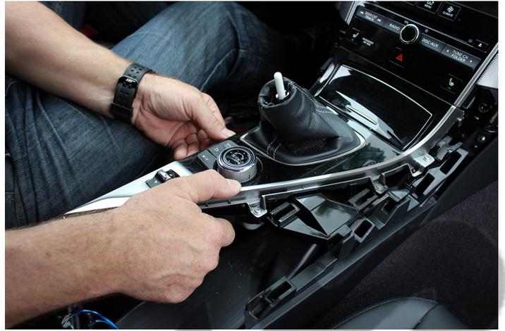
Unfasten **four (4)** screws securing shifter / center console trim panel.
