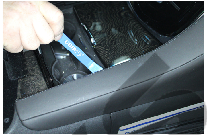
Pry out passenger side center console trim panel.
