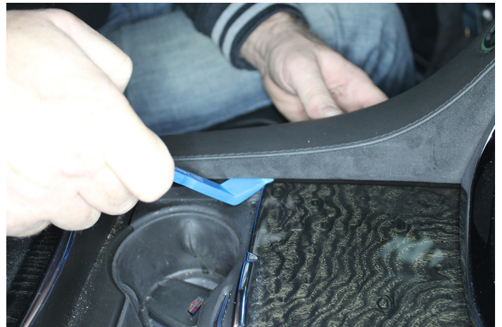
Pry out driver side center console trim panel. Disconnect start button plug.
