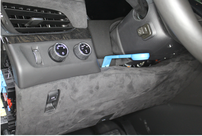
Pry out steering wheel column cover. Disconnect two (2) plugs: park switch, hood latch.
