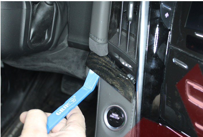
Pry out steering wheel column cover. Disconnect two (2) plugs: park switch, hood latch.
