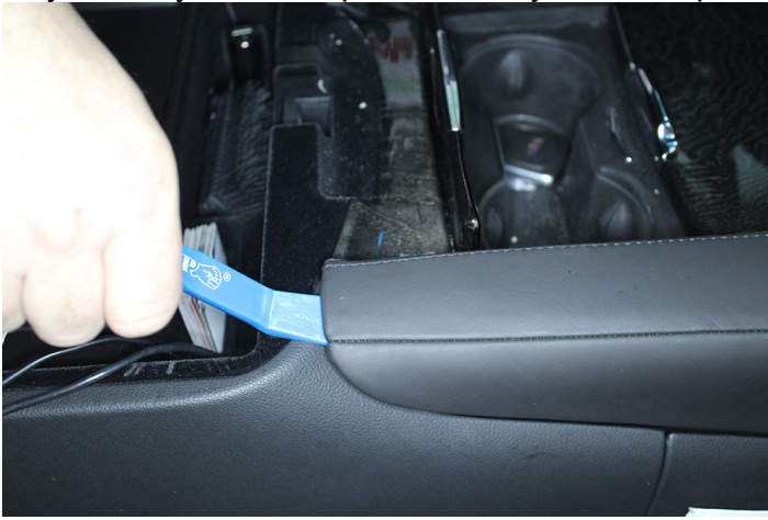
Pry out passenger side center console trim panel.
