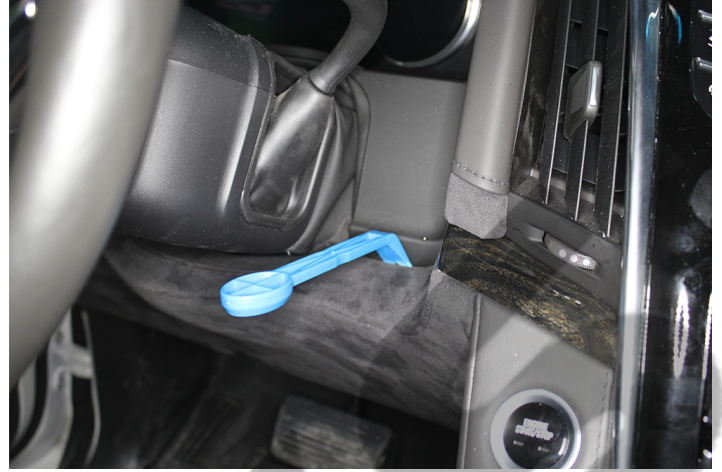
Pry out steering wheel column cover. Disconnect two (2) plugs: park switch, hood latch.
