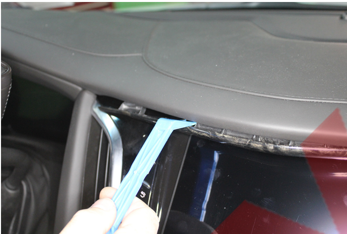
Carefully pry out trim bezel between the screen and the dash.
