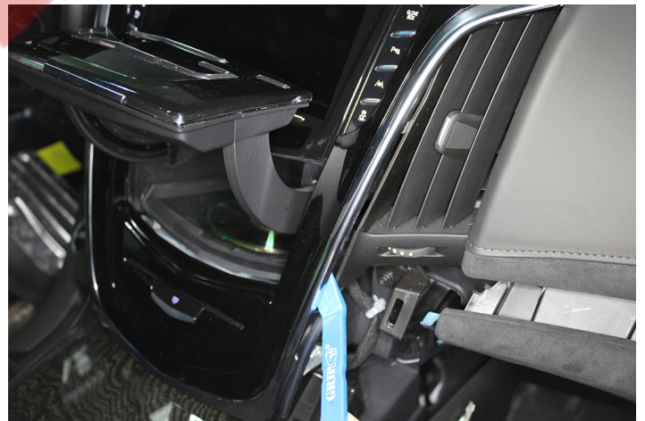
Pry out silver radio bezel to expose radio unit screws. Work your around both sides top to bottom.
