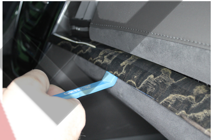
Pry out steering wheel column cover. Disconnect two (2) plugs: park switch, hood latch.
