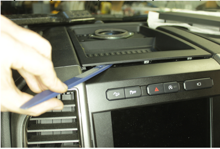
Pry out top trim panel to expose two (2) screws above the screen. Disconnect one (1) plug and remove speaker panel.
