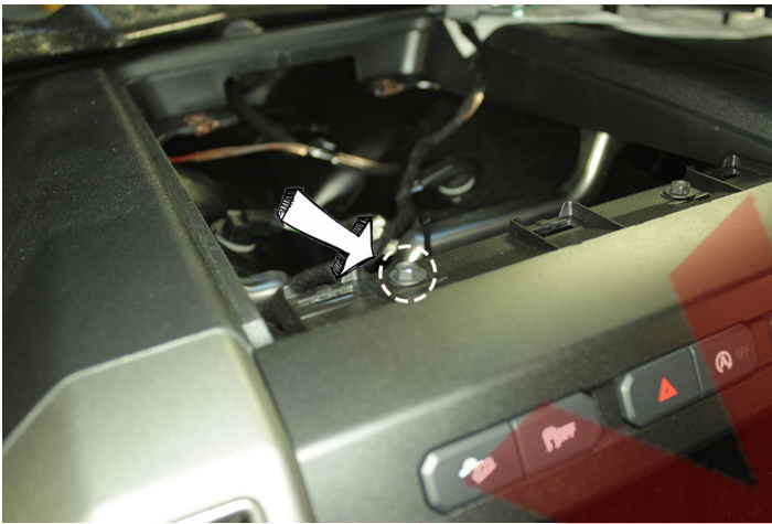
Unfasten two (2) screws securing the dash trim bezel.
