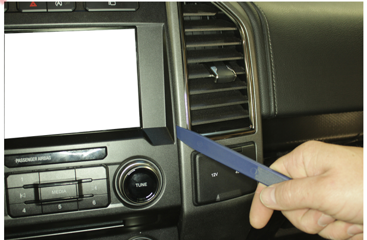
Starting at the top of the dash trim bezel using a panel prying tool pry out dash trim bezel.
