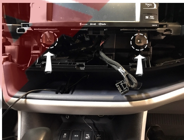
Unfasten two (2) bolts under the radio unit. Slide radio out slowly.
