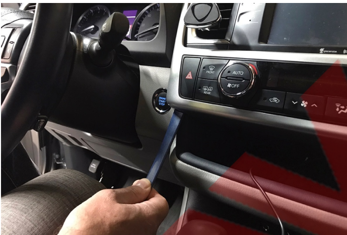
Pry out climate control trim panel, disconnect two (2) plugs.
