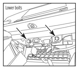
Unfasten four (4) screws, two (2) atop of s screen head unit and two (2) at the bottom.
