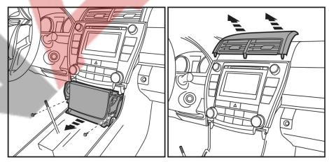
Pry out pocket under the radio unit. Pry out air vents on top of the screen.
