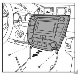
Unfasten four (4) bolts: two (2) atop the radio and two (2) under the radio.
