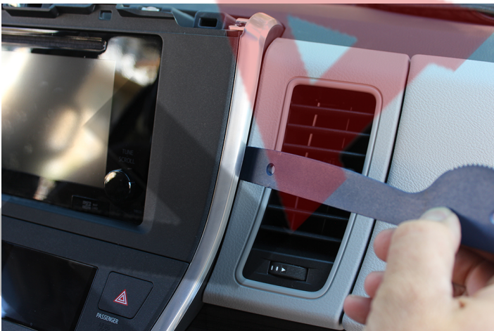
Pry out climate control / screen trim panel. Gently pull to remove it, disconnect two (2) plugs.
