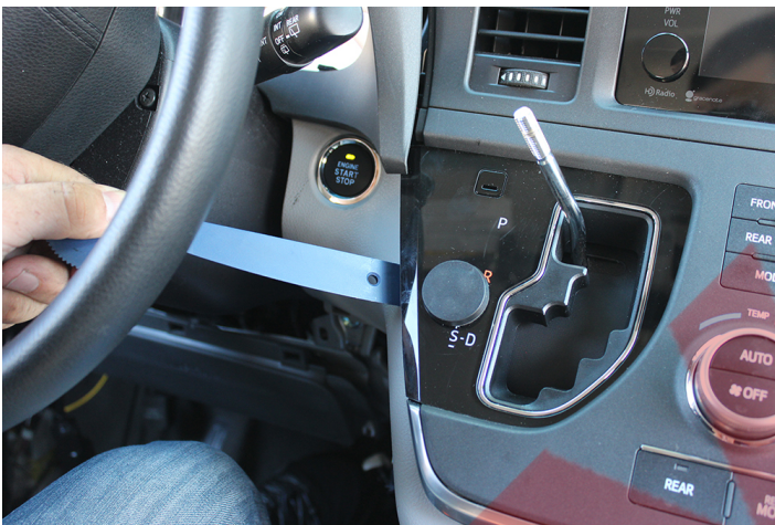
Unfasten gearshift knob. Pry out climate control / screen trim panel.
