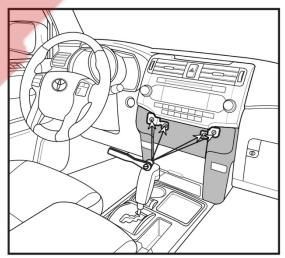
Unfasten **four** (**4**) bolts under the radio. Pull radio unit out slowly.
